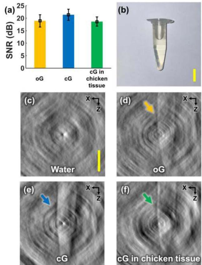
**Fig. 2.** (a) SNRs versus various Gastrografin conditions. (b) Photograph of material in the e-tube. Cross-section XACT images of (c) water, (d) oG, (e) cG, and (f) cG in chicken tissue. The yellow scale bar is 10 mm. Chicken tissue size is  $28 \text{ mm} \times 28 \text{ mm} \times 40 \text{ mm}$  [width (X)  $\times$  length (Y in Fig. 1)  $\times$  height (Z)].
