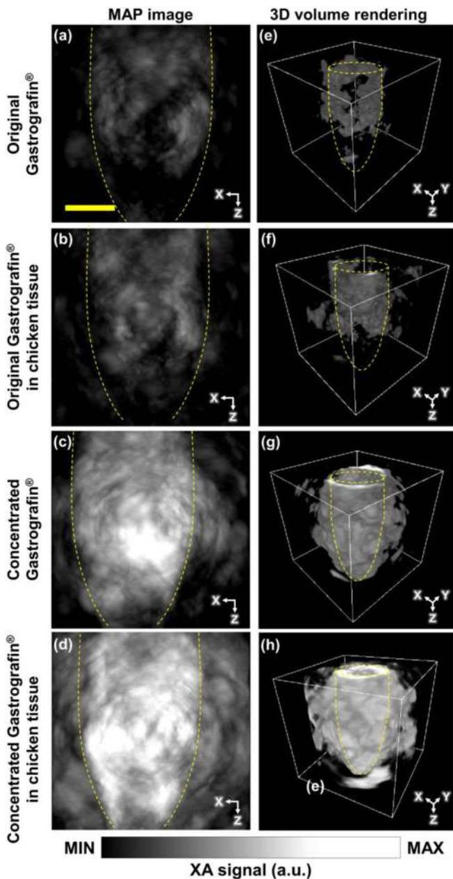
**Fig. 3.** (a)–(d) Two-dimensional MAP XACT images and (e)–(h) 3D volumetric rendering of various phantoms. The yellow scale bar is 10 mm. Chicken tissue size is 28 mm × 28 mm × 40 mm (width × length × height).
