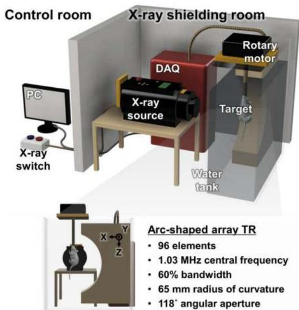
**Fig. 1.** Schematic of XACT system: TR, transducer; DAQ, data acquisition board.
