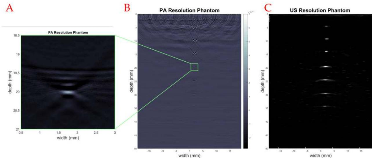
Figure 6: PA spatial resolution phantom image with “bone” colormap, US with greyscale colormap. A zoomed portion of the PA reconstruction with modified dynamic range was analyzed for spatial resolution (A). The full PA phantom depth (B). The full US phantom depth (C).
