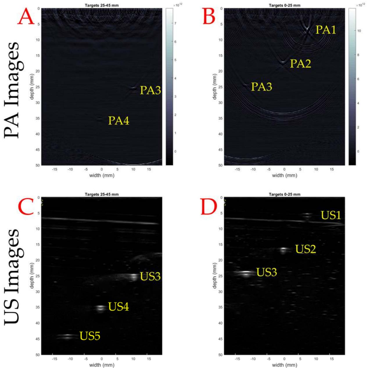
Figure 7: Depth sensitivity phantom. The PA reconstruction images of the depth sensitivity phantom at two height windows (A, B). The US reconstruction images of the depth sensitivity phantom at two height windows (C, D). The detected microcuvettes filled with samples are labeled as PA/US (1, 2, 3, 4, 5).
