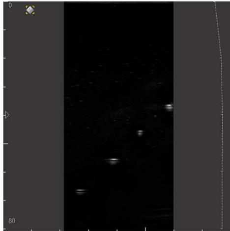
Figure 8: US image of depth sensitivity phantom, phantom height window 35 – 65 mm, full depth scale from 0 – 80 mm.
