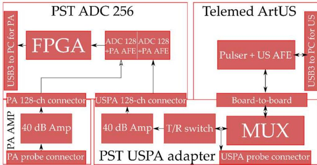
Figure 2: Block-diagram of the USPA device's subsystems.
