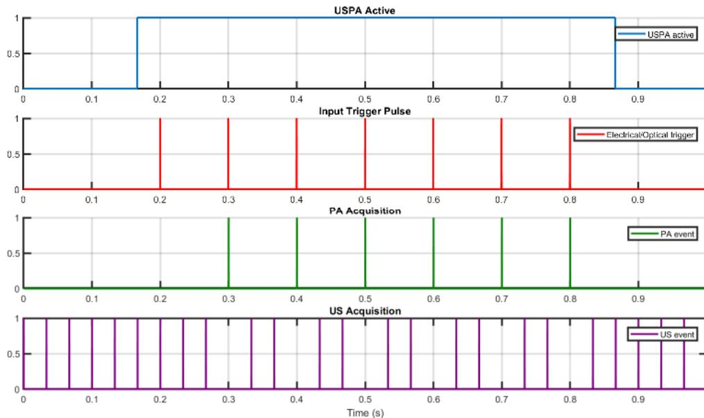
Figure 3: Timing diagram of the USPA system's communication. Example with 10 Hz laser, US continuous mode.
