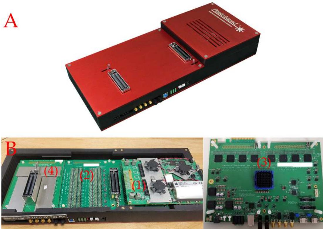
Figure 1: MolecuUS system in housing (A). MolecuUS system without housing (B); USPA adapter board (1), US device (2), PA pre-amp board (3), PA ADC (4).
