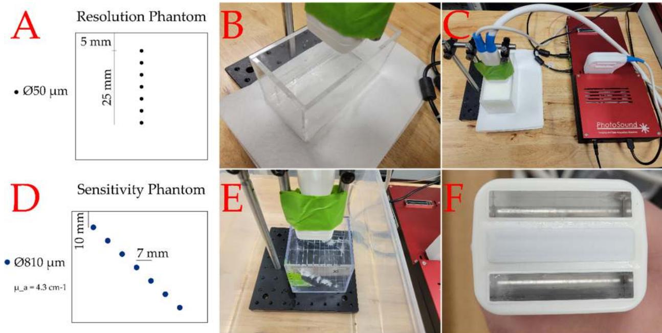
Figure 4: Phantom experiment setup. Spatial resolution phantom diagram (A), spatial resolution phantom setup (B), full imaging setup, except for the laser (C), depth sensitivity phantom diagram (D), depth sensitivity phantom setup (E), probe face with detector array and fiberoptic outputs (F).
