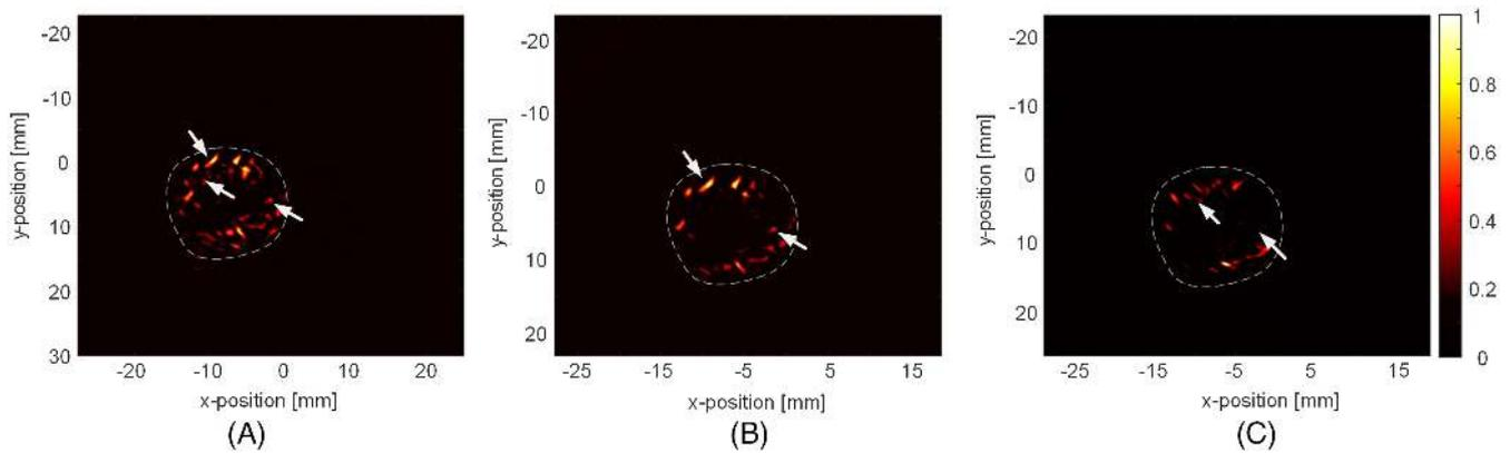
**FIGURE 14** The human finger imaging results with multiple frequencies reconstruction. (A) the imaging result with multiple frequency PA signals; (B) the imaging result with low frequency (center frequencies are 1 and 2.5 MHz) PA signals; (C) the imaging result with high frequency (center frequencies are 5 and 7.5 MHz) PA signals (the white dashed line marks the surface of skin)
