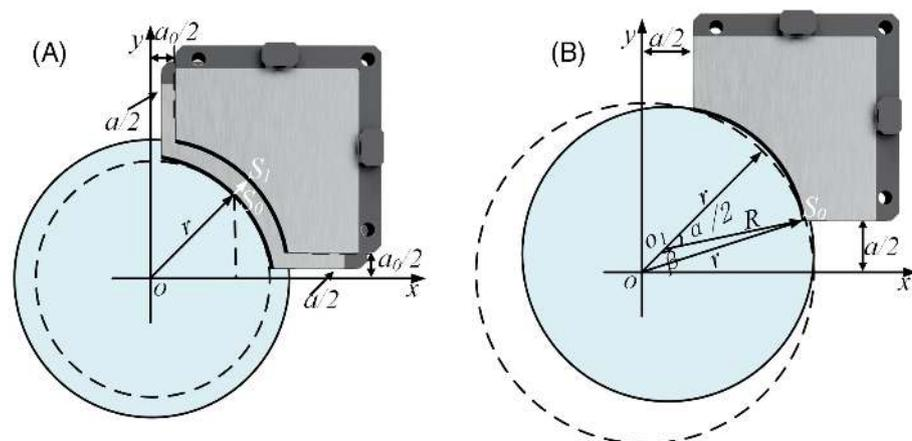
FIGURE 4 The radius of the inscribed circle calculation model for the ROI of the SUTA-based PAT system. (A) the SUTAs for the small region for signals detection ( $0 \leq a \leq a_0$ ),  $o$  is the center of the imaging region,  $S_0$  is the tangent point of the small imaging region circle to the SUTA arc; (B) the SUTAs formed a large region for PA signals detection ( $a \geq a_0$ ),  $o$  is the center of the large imaging region,  $o_1$  is the center of the SUTA arc
