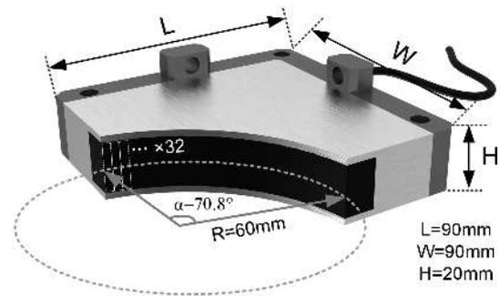
FIGURE 2 The proposed SUTA schematic diagram. L, length; W, width; H, height; R, radius
