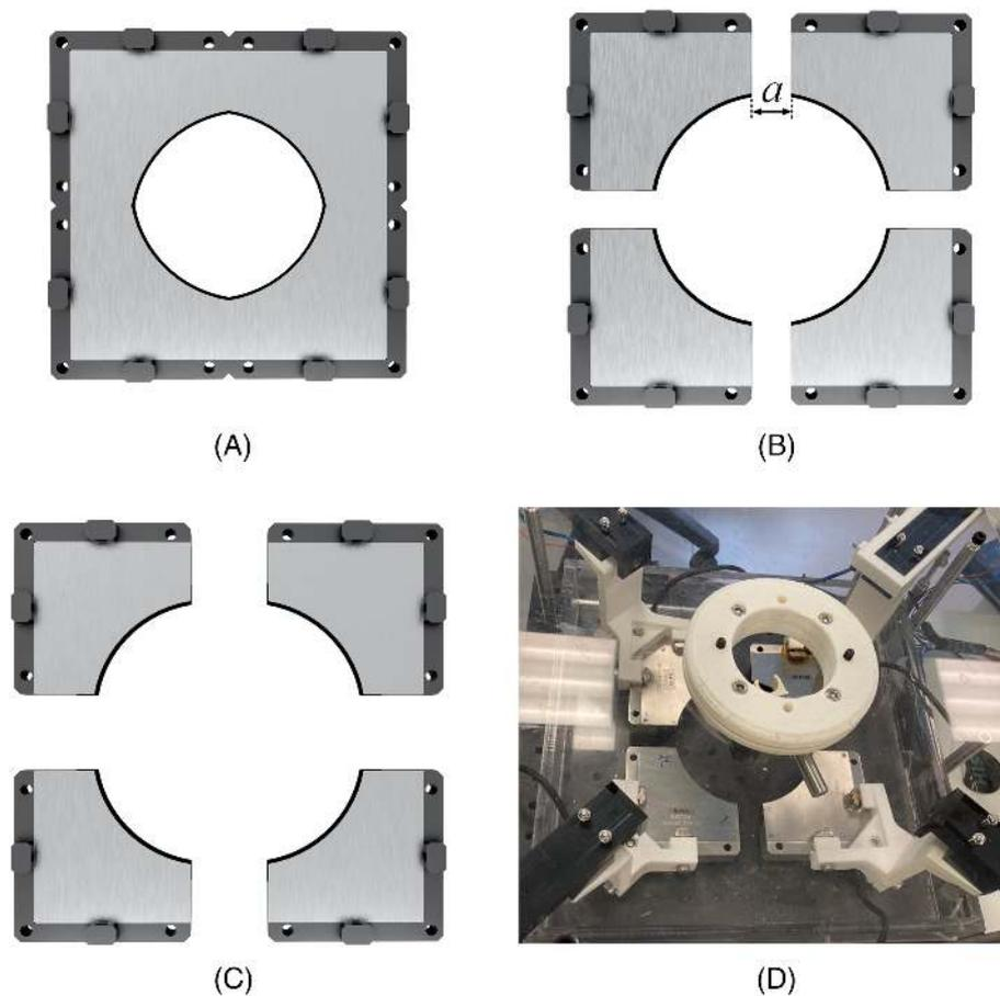
FIGURE 3 The ROI size-adjustable PAT system with four SUTAs. (A) is the situation for small ROI with 50 mm radius, (B) forms a middle size region with 60 mm radius and (C) is for large ROI; (D) the photograph of the four SUTAs' distribution controlled by stepper motors
