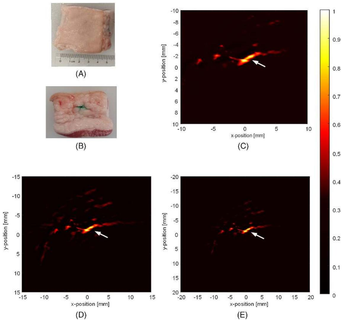
FIGURE 12 The ex-vivo imaging results. (A) the photograph of the pork breast; (B) the lateral view of the pork breast with ICG injections; (C–E) the imaging results with various sizes of imaging region corresponding to  $20 \times 20 \text{ mm}^2$ ,  $30 \times 30 \text{ mm}^2$  and  $40 \times 40 \text{ mm}^2$  view, respectively; the white arrow indicating the injected ICG
