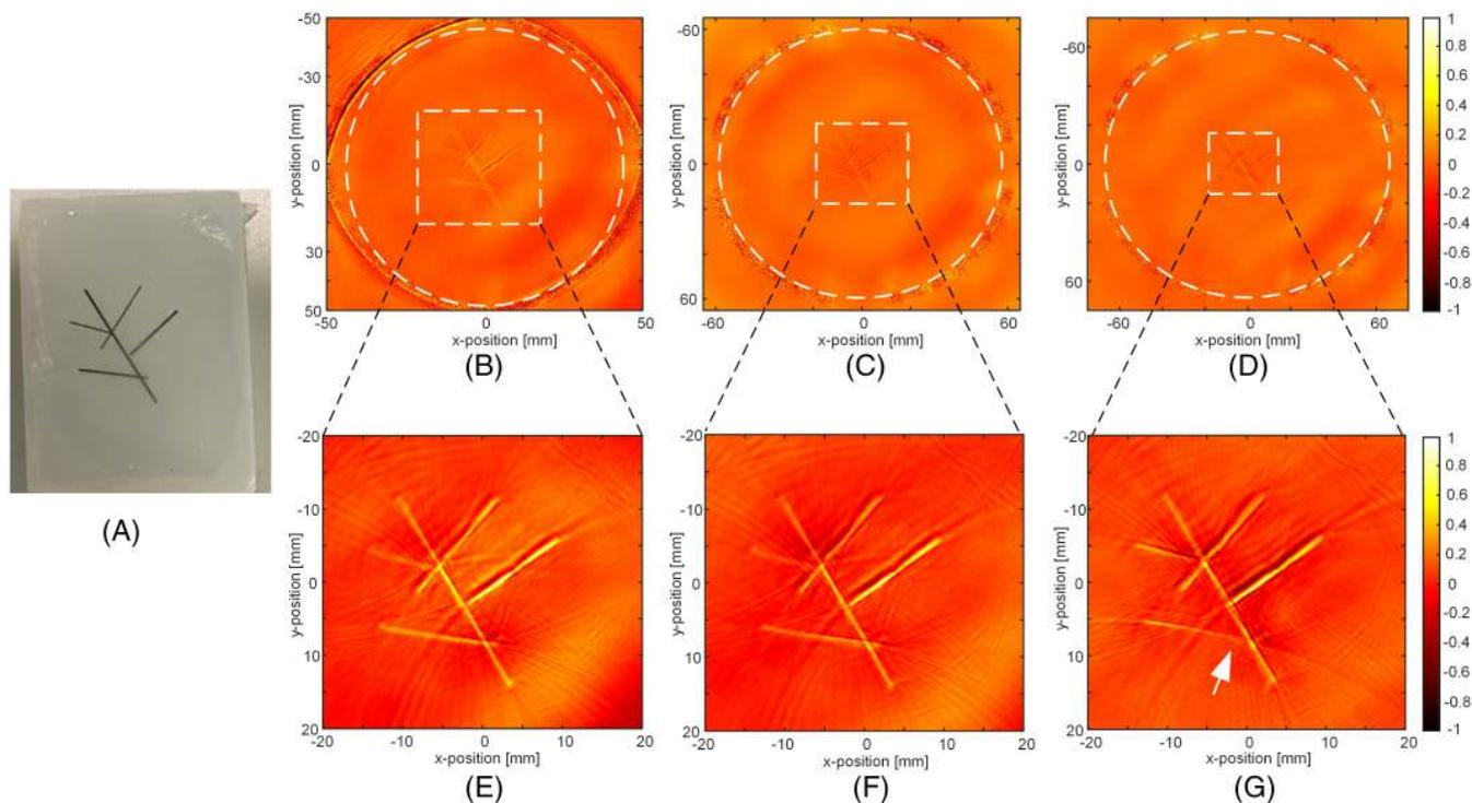
**FIGURE 11** The phantom imaging results. (A) the photograph of the phantom; (B), (C) and (D) are the top view of imaging results corresponding to  $a = 0$  mm,  $a = 20$  mm and  $a = 35$  mm with different imaging sizes; (E), (F) and (G) are the region of interest of the imaging results corresponding to the (B), (C) and (D), respectively
