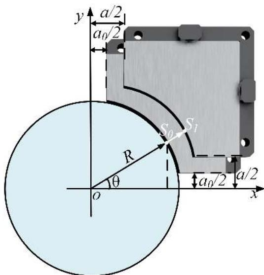
**FIGURE 6** The coordinate calculating model for the first quadrant SUTA's transducer elements.  $\theta$  is the angle of the transducer element,  $S_0$  is the element position with  $a = a_0$  and  $S_1$  is the element that needs to be calculated. (The four SUTAs are arranged in the four quadrants, respectively; the original point is defined in the center of the imaging area)
