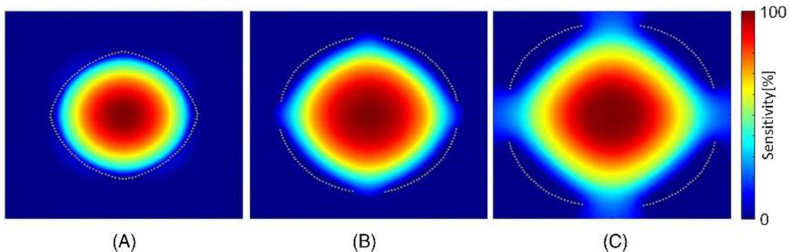
FIGURE 9 The simulated sensitivity map of various distribution of the SUTAs. (A), (B) and (C) stand for the small, middle and large field of view scanning schemes, respectively (parameter  $a = 0, 20$  and  $40$  mm)
