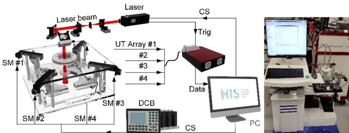
FIGURE 10 The proposed size-adjustable PAT system setup and its photograph. #, device number; CS, control signal; DCB, digital control board; PC, personal computer; SM, stepper motor; Trig, trigger; UT, ultrasound transducer
