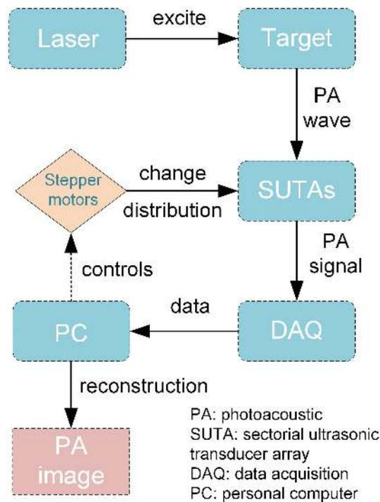
FIGURE 1 The overview of the size-adjustable PAT system workflow
