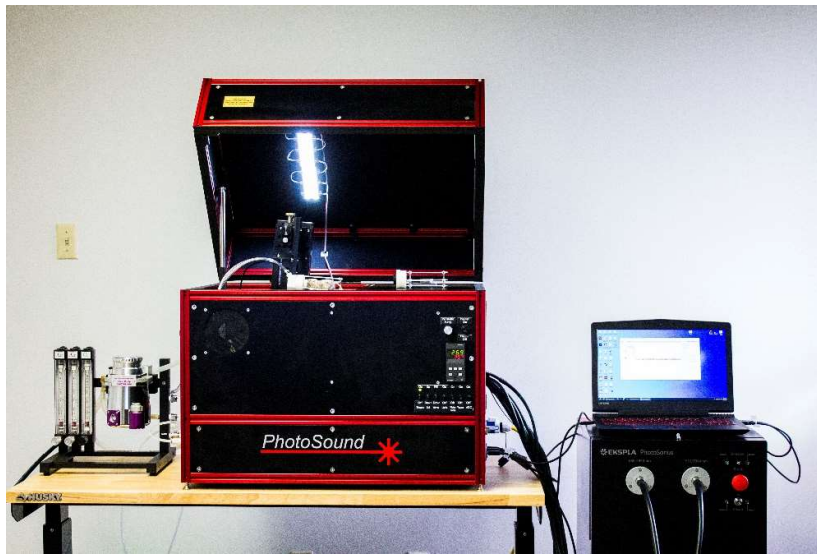
Custom Real-time PhotoAcoustic Tomography Platform designed by PhotoSound®
