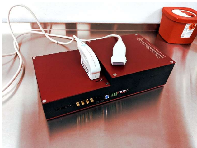
PhotoSound® MoleculUS™, ultrasonic imaging with molecular analysis
