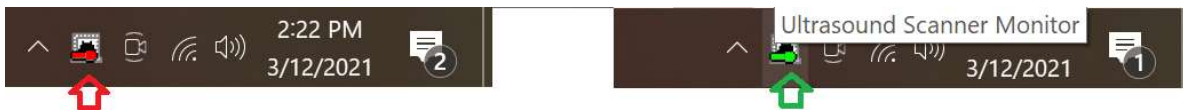
Figure 30: Ultrasound Scanner Monitor indicating the connection status of the ArtUs device to the PC. Red – not connected or/and no power; green – powered, connected and ready.
