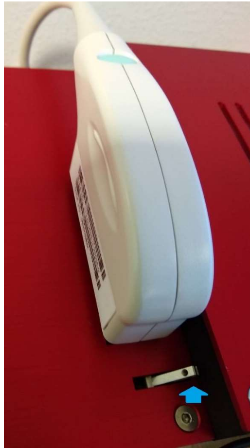
Figure 7: A probe plug is inserted into the USPA socket and the latch is closed. The PA-only connection is similar.
