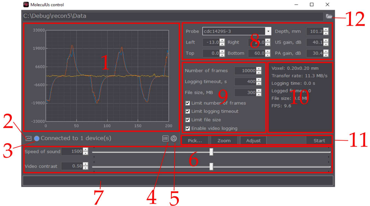
Figure 33: MoleculUS control main window Main control hub of the MoleculUS's PA signal acquisition and reconstruction. Digital oscilloscope (1), plot control (2), status bulb (3), Capture and trigger settings (4), Configuration menu (5), speed of sound and contrast sliders (6), capture progress bar (7), real-time reconstruction settings (8), capture parameters (9), status monitor (10), action buttons (11), folder button (12), real-time reconstruction viewer (13).
