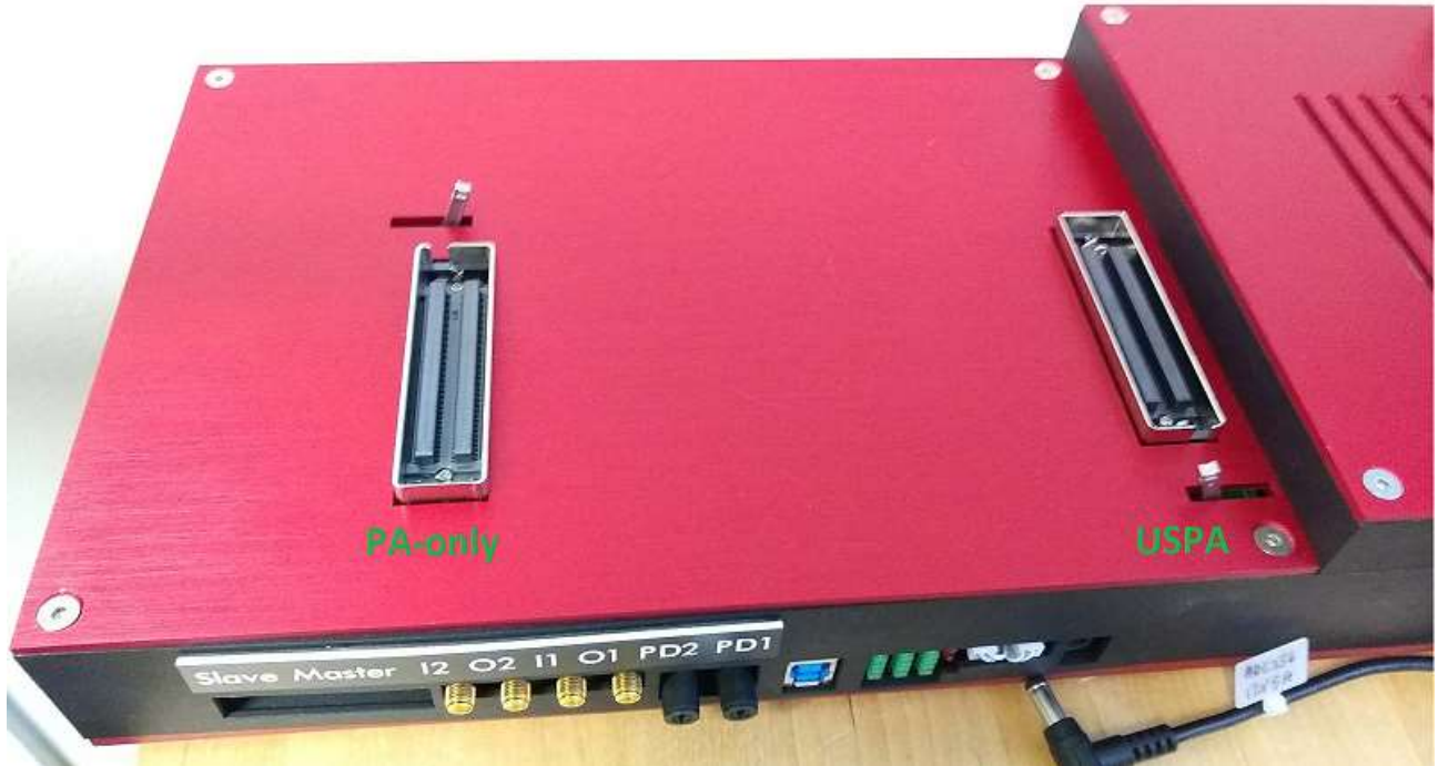
Figure 5: Plug a US probe into the USPA connector. Plug a PA-only probe into the PA-only connector. A PA type of connector can be customized.
