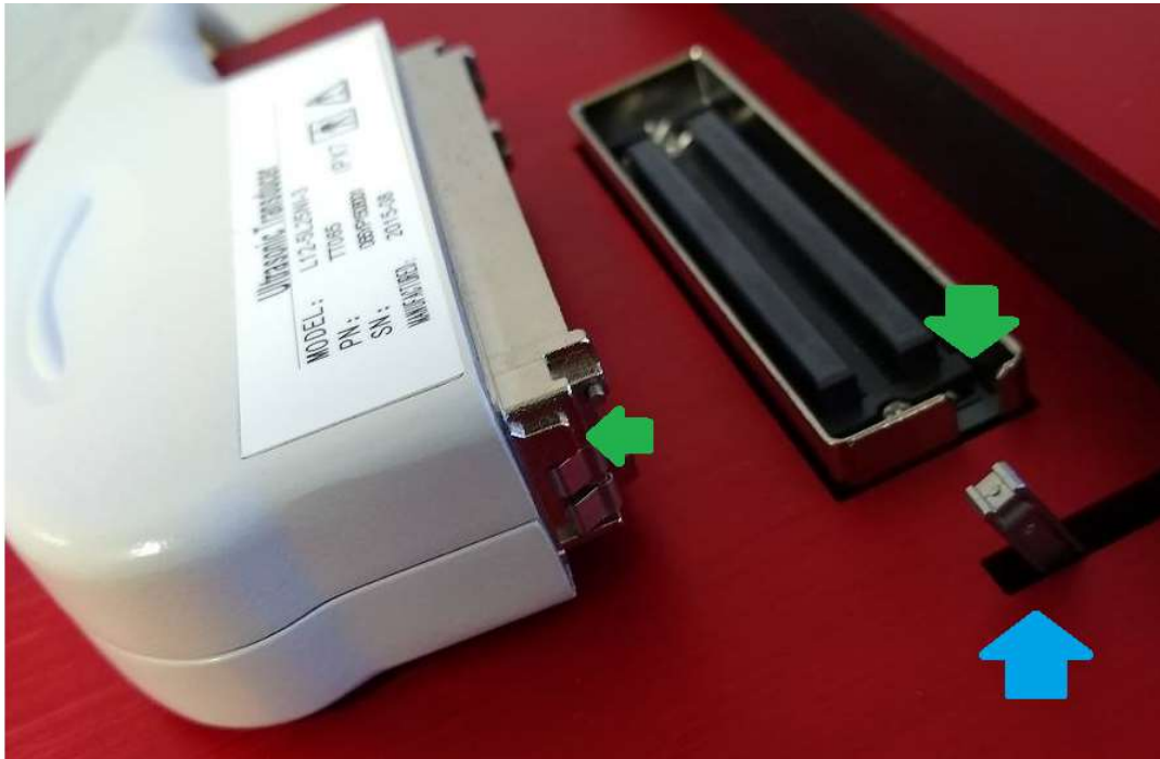
Figure 6: The probe plugs and sockets have alignment keys, as indicated by the green arrows. The probe sockets have latches, as indicated by the blue arrow.
